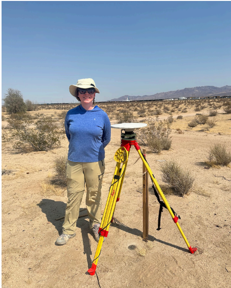
Figure 2: SCEC SURE intern Katie Baraggiota, standing by a completed GNSS antenna set-up.
