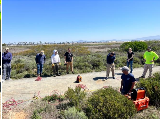
Fig. 4: Photos from the Advanced Field classes collecting resistivity and seismic reflection data in the TRNEER.
