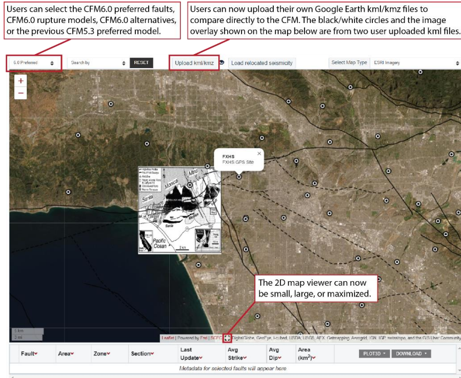
Figure 3: View of the updated CFM web tools zoomed to the Los Angeles region with new features highlighted with red outlined text boxes. The view above shows two kml/kmz files loaded. The circles show locations of permanent GPS stations. The image overlay is a map from Dolan & Pratt (1997) of the Santa Monica Mountains regional geology. Allowing users to upload their own kml files allows for direct and easy comparison of user data to the CFM and should be useful for other SCEC community models in the future.
