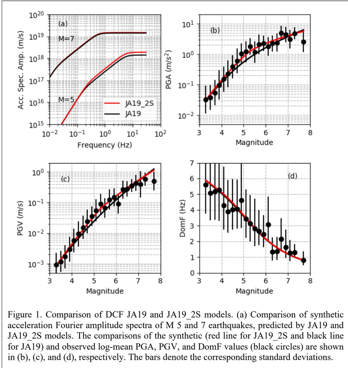
Figure 1. Comparison of DCF JA19 and JA19\_2S models. (a) Comparison of synthetic acceleration Fourier amplitude spectra of M 5 and 7 earthquakes, predicted by JA19 and JA19\_2S models. The comparisons of the synthetic (red line for JA19\_2S and black line for JA19) and observed log-mean PGA, PGV, and DomF values (black circles) are shown in (b), (c), and (d), respectively. The bars denote the corresponding standard deviations.
