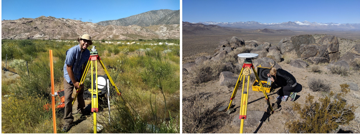
Figure 1: Examples of data collection. Left: SURE intern Eneas Torres-Andrade, leveling a GPS tripod at site G036 in the Cajon Pass area in June 2018. Right: Graduate student Rachel Terry, setting up a GPS receiver at site PASO, SE of Ridgecrest in February 2019.
