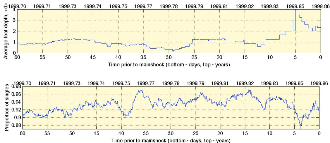
**Figure 2:** Premonitory changes of clustering prior to Duzce mainshock, 12 November 1999, M7.1. Top panel: Average leaf depth  $\langle d \rangle$  in a moving window of 7 days for families with mainshock magnitude  $m > 3$ . Bottom panel: Proportion of singles among all the clusters in a moving window of 3 days.
