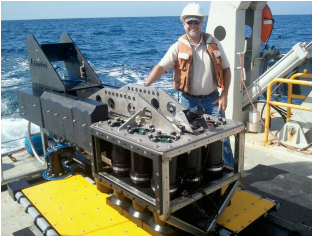
Figure 1. SAS CHIRP is shown with cowling removed. The nine tonpilz transducers are mounted in the bow of the vehicle. The two retractable yellow wings with the receiving arrays are controlled by the cylindrical motors near the aft of the vehicle.
