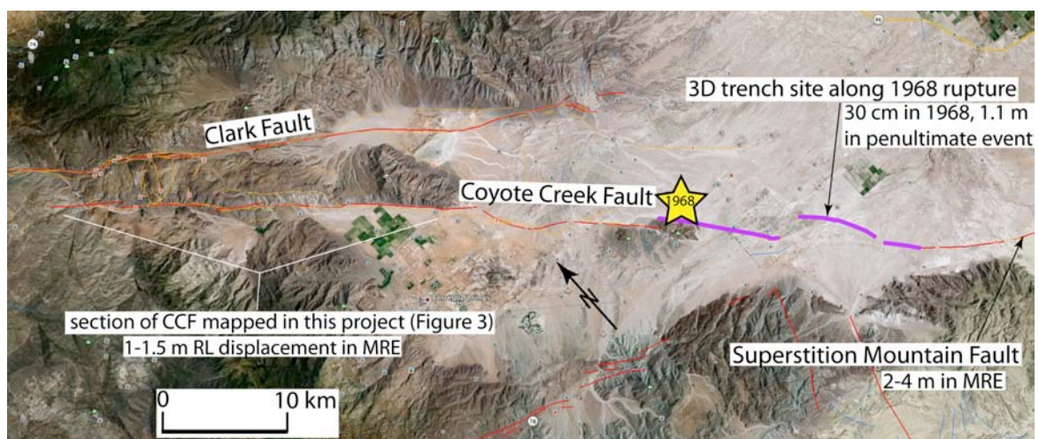
Figure 2. Detail of mapped area on GoogleEarth base image. The slip distribution interpreted from our mapping is shown in figure 3. The results of the 3D trenching are shown in figure 4
