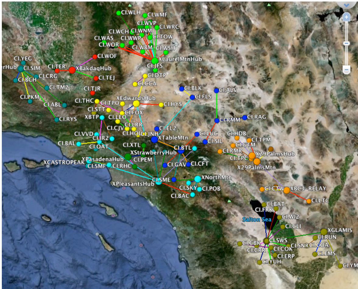
Figure 1. Example of telemetry path information stored in Station Information System (SIS). SCSN Telemetered Short Period Stations.
