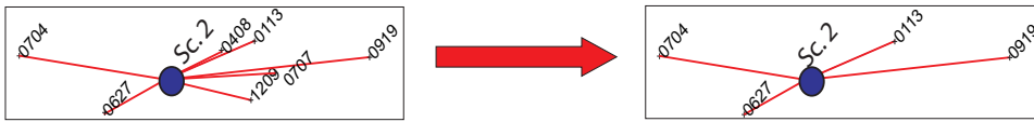
Figure 1: Partial elimination of interferograms that cancels a contribution of a “noisy” SAR scene.
