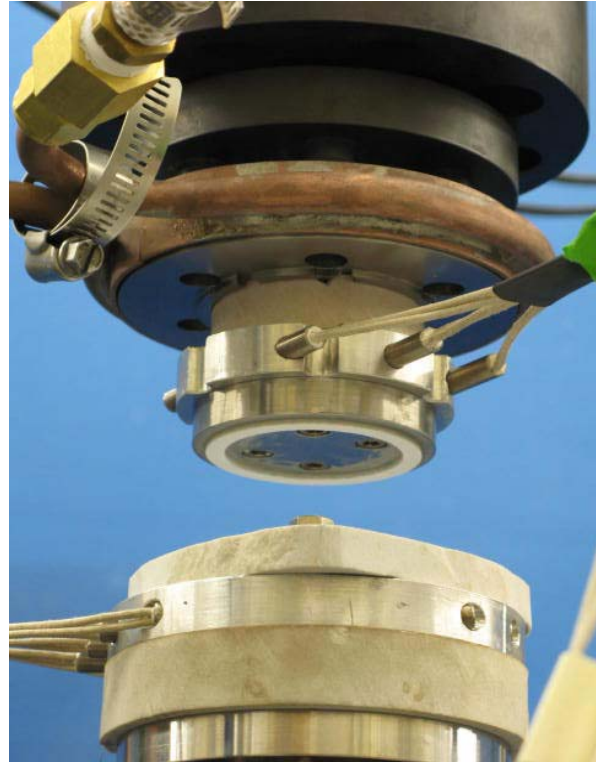
Figure 3 – Photographs of the high temperature sample assembly mounted in the Instron torsion/compression load frame. Aluminum blocks above the upper sample ring and the lower sample plate (novaculite sample shown) are heated with cartridge-type resistance heaters. Temperatures will be monitored with thermocouples embedded in the sample surface. Copper cooling jacket on upper sample grip, with flowing water inside the jacket, protect the load and torque cell from overheating. Preliminary tests indicate that temperatures in excess of 300 °C are easily obtained.
