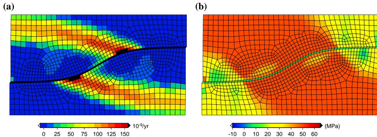
**Figure 1:** (a) Square root of the second (shear) invariant of the deviatoric strain-rate tensor at 5 km depth. Colors show off-fault strain rate (nano-strain/yr), shear strain within the fault zone is off-scale and would dominate the plot. (b) Square root of the second invariant of the deviatoric stress tensor at 5 km depth.
