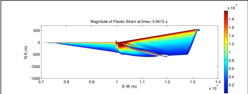
Figure 3. The distribution of off-fault plastic strain magnitude in the elastoplastic calculation of the kinked fault. Distinct features are associated with the fault kink.
