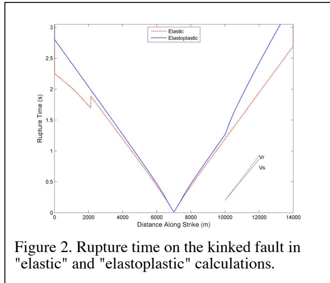
Figure 2. Rupture time on the kinked fault in "elastic" and "elastoplastic" calculations.
