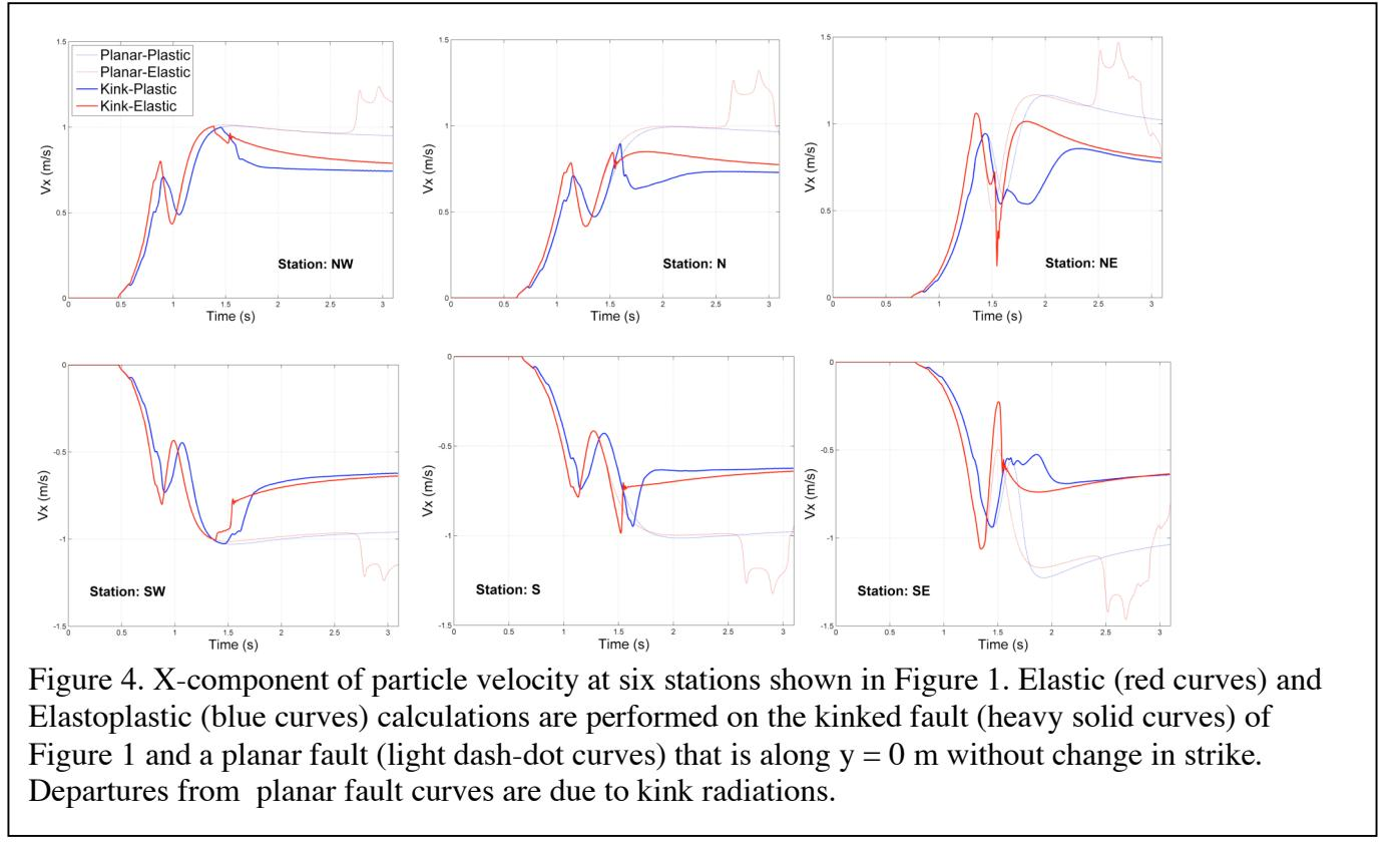
Figure 4. X-component of particle velocity at six stations shown in Figure 1. Elastic (red curves) and Elastoplastic (blue curves) calculations are performed on the kinked fault (heavy solid curves) of Figure 1 and a planar fault (light dash-dot curves) that is along  $y = 0$  m without change in strike. Departures from planar fault curves are due to kink radiations.
