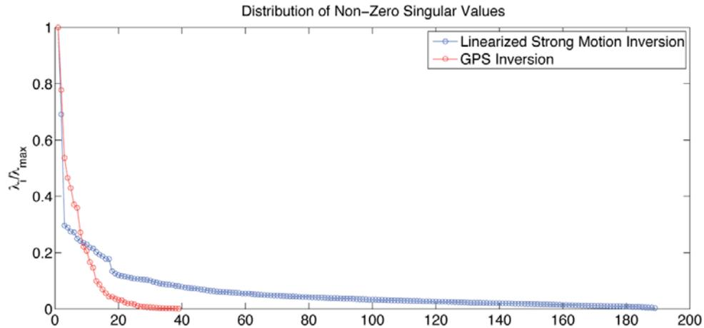
**Figure 5.** Distribution of singular values for the GPS inversion (red) and for a linearized strong-motion inversion (blue). The strong-motion inversion is not technically underdetermined, although many of the singular values are near zero, which means some slip vectors are unstable.
