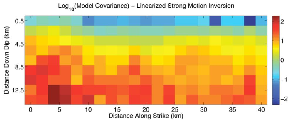
**Figure 6.** The model covariance, which shows how sensitive model parameters are to perturbations in the data, is shown plotted onto the fault plane for a linearized strong-motion inversion.
