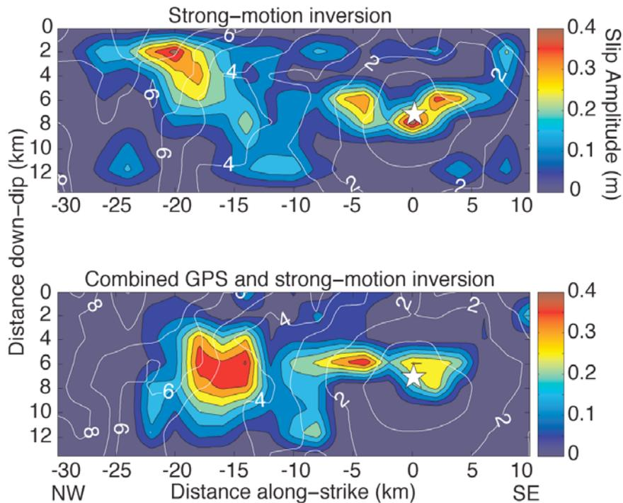
**Figure 4.** Inversion of strong-motion GPS data without any static-field constraint [Liu *et al.*, 2006] (a), and with the addition of a final-slip constraint derived from the GPS data inverted on a nonuniform grid (b). The addition of GPS data results in a more compact final slip distribution.
