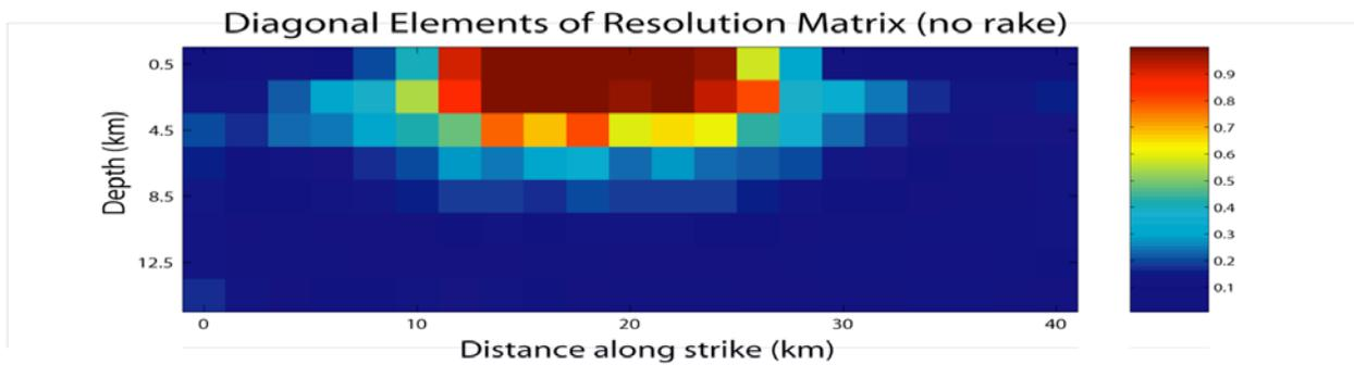
**Figure 1.** Diagonal elements of the resolution matrix for the GPS data from the 2004 Mw6.0 Parkfield Earthquake plotted on their corresponding subfaults. Resolution is poor at depth and near the edges of the fault.
