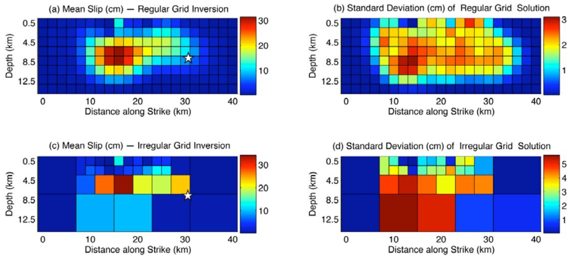
**Figure 3.** Inversion of Parkfield GPS data on a regular grid (a), and on an irregular grid (c), with associated perturbation errors found via Monte Carlo sampling of GPS errors (b and d). Both inversions give similar fits to the data with a variance reduction of 89-90%.
