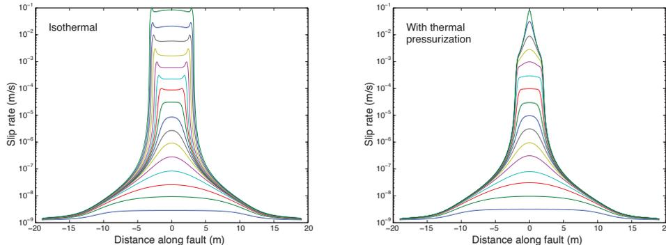
Figure 1: Slip-rate profiles at different snapshots in time comparing isothermal case (left) with thermal pressurization (right). Aging law,  $a/b = 0.8$ ,  $a = 0.015$ ,  $d_c = 100\mu\text{m}$ , and  $\sigma - p^\infty = 140$  MPa.  $c_{hyd} = 8 \times 10^{-6} \text{ m}^2/\text{s}$ .
