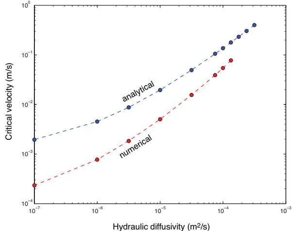
Figure 2: Comparison of analytical (8) and numerical estimates of  $v_{crit}$ , the critical slip speed beyond which thermal pressurization dominates over frictional weakening.  $d_c = 100\mu\text{m}$ ,  $\sigma - p^\infty = 140$  MPa, and  $a/b = 0.8$ .
