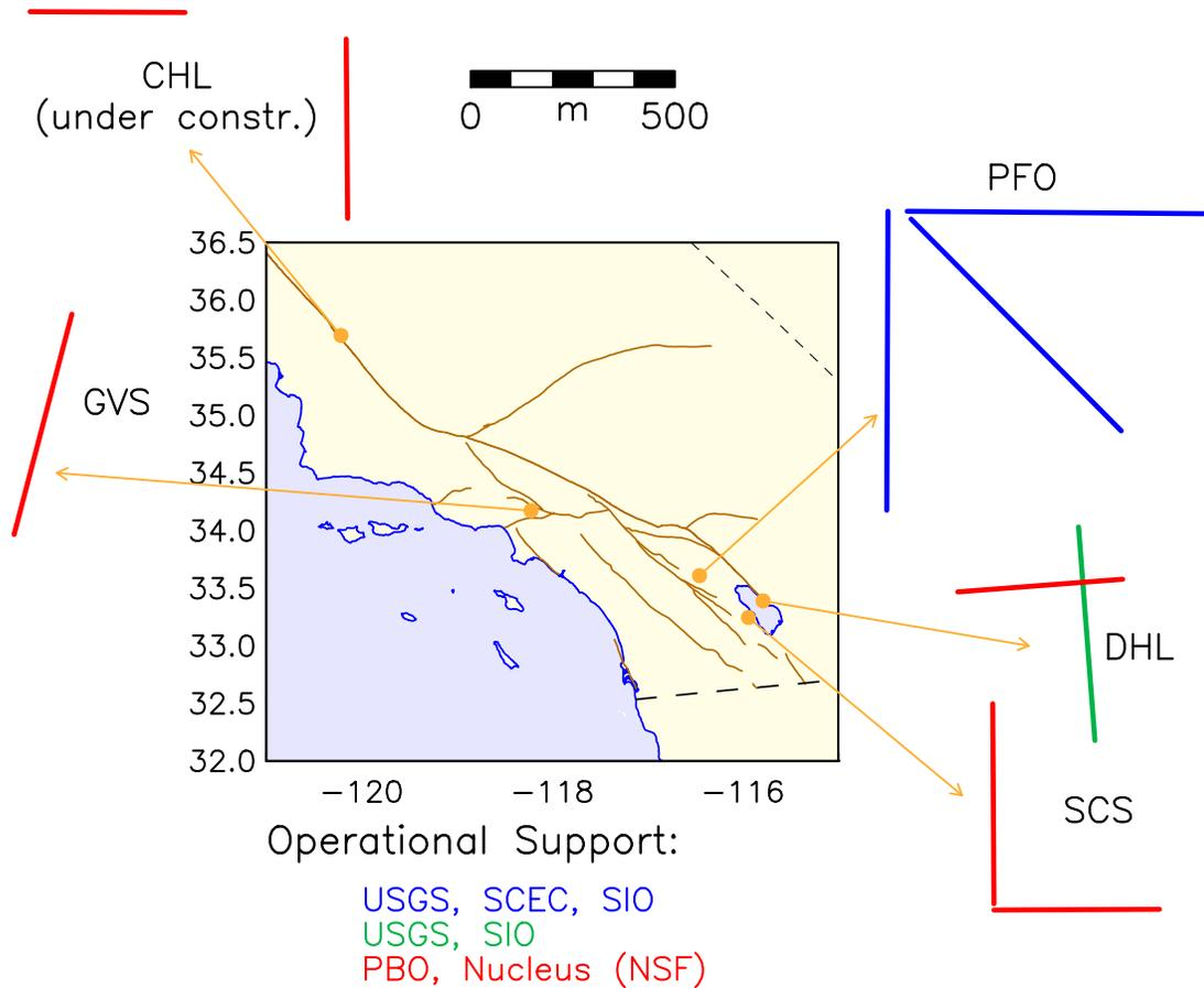
Figure 1: Laser strainmeters in California. All of the systems are telemetered by radio links and Internet to UCSD, with data streamed, and also downloaded daily.
