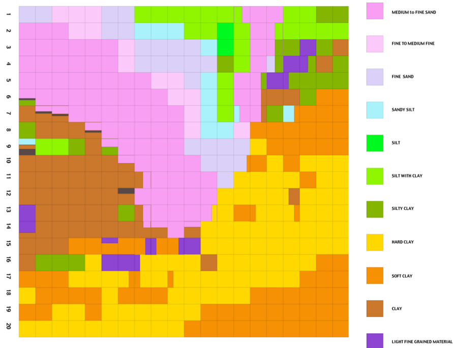
Figure 13. Image based on the samples descriptions. The boundaries of the clays units shown in Figure 8 were not always observed when describing individual samples.
