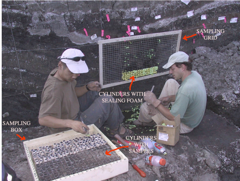
Figure 3: North wall of trench T-2 were the box, grid and samples can be seen.
