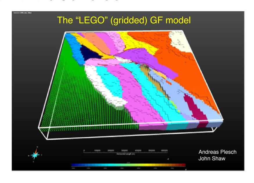
Grid cell dimensions are 10 km x 10km x 1km. Depth of volume is 60km, will extend to 80+ km. Geo-referenced surfaces will include topography/bathymetry, sediment-basement boundary, bottom of seismogenic crust, Moho, and lithosphere/asthenosphere boundary. Lithology contact surfaces are defined within provinces.
