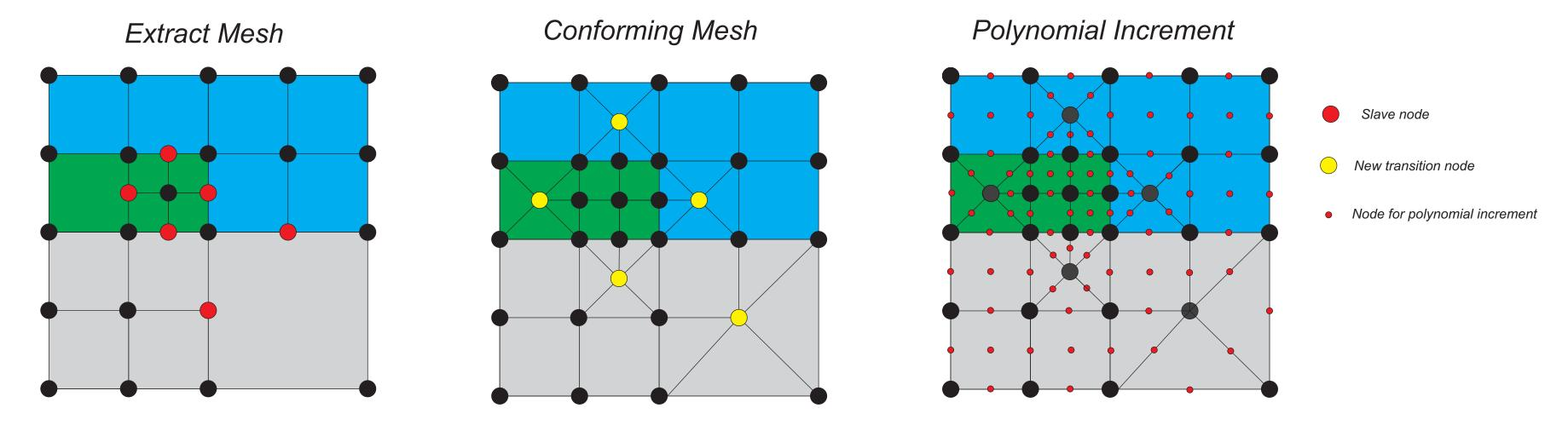
Figure 1. Octree structure and domain meshing approach. A) Extract mesh. B) Identify transition elements and add a new node to generate additional elements. C) Addition of degrees of freedom
