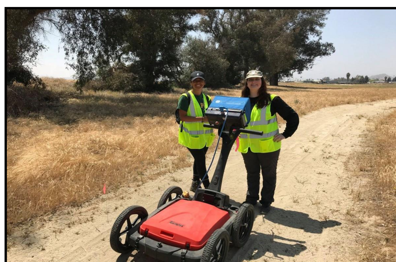
Figure 3 (left): Ground Penetrating Radar survey at the Pellissier Ranch site.
