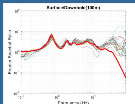
Figure 3. Comparing spectral ratios obtained from shstack (thick red) with those obtained from recorded data, at 100m depth (similar plots are developed for other 4 downhole depths also)
