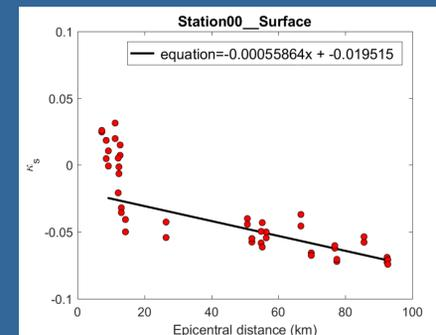
Figure 5. kappa versus epicentral distance plot  $\kappa_s$  derived from recorded events (similar plot is developed for  $\kappa_p$  also)
