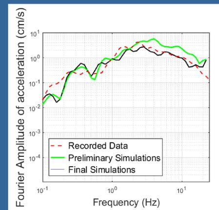
Figure 8. Comparison of Fourier amplitude spectrums for final and preliminary simulations with that of recorded earthquake event (N-S component)
