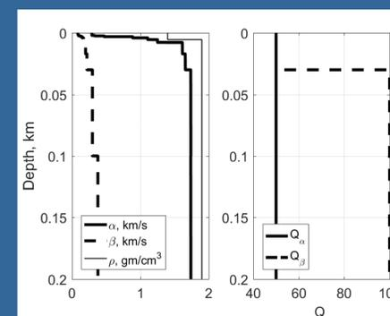
Figure 6. Final velocity and Q-profiles in the upper 200m
