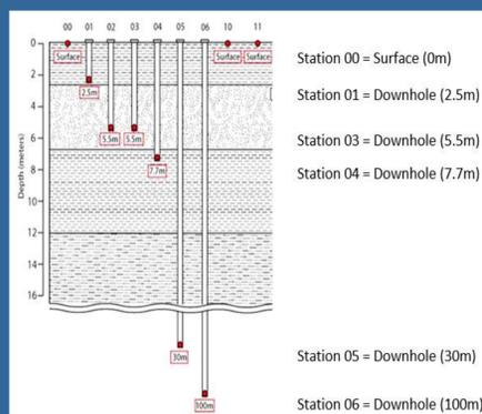
Figure 1. Representation of Depths (vertical) and Station-IDs (horizontal) of accelerometers at WLA, adopted from NEES@UCSB website
