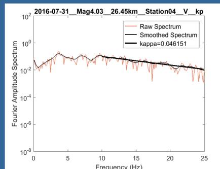
Figure 2. Calculation of kappa from an acceleration spectrum
