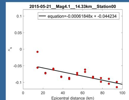
Figure 7. kappa versus epicentral distance plot  $\kappa_s$  derived from 12 station simulations
