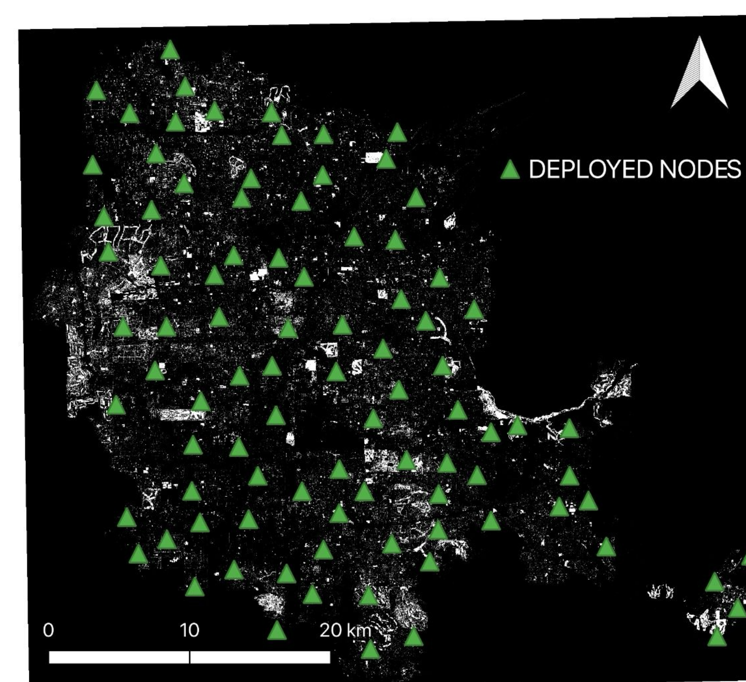
Figure 2B - Early June 2025, We deployed 91 of 106 available seismometers. They were retrieved ~30 days later [2](Poster #020).
