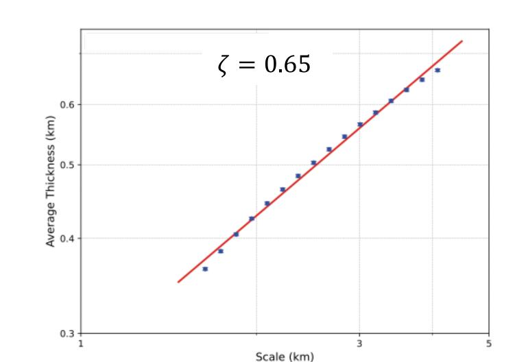
The apparent thickness increases with scale, following a power-law relationship:  $h(r) \propto r^{\zeta}, 0 < \zeta < 1$
