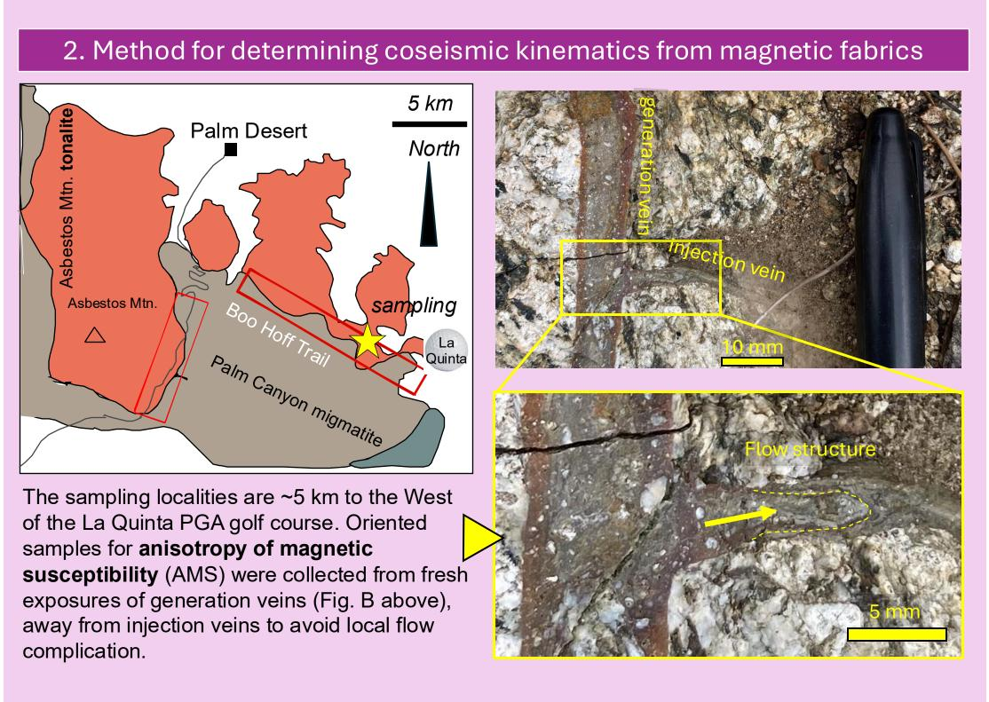
Slabs (3.5 mm thick) were cut along the horizontal plane and cubes were cut from these slabs along NS and EW vertical directions. The mini-cubes (3.5 mm) are measured using custom-made diamagnetic acrylic holders in a Kappabridge, KLY-5S susceptometer.
