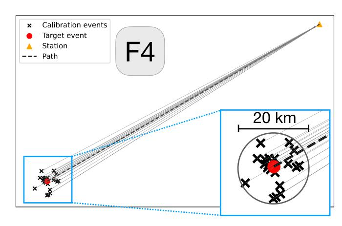
F4: Station and path corrections using small, nearby calibration events. This is analogous to the spectral decomposition method in Shearer et al. (2022), where  $f_c$  of calibration events are fixed
