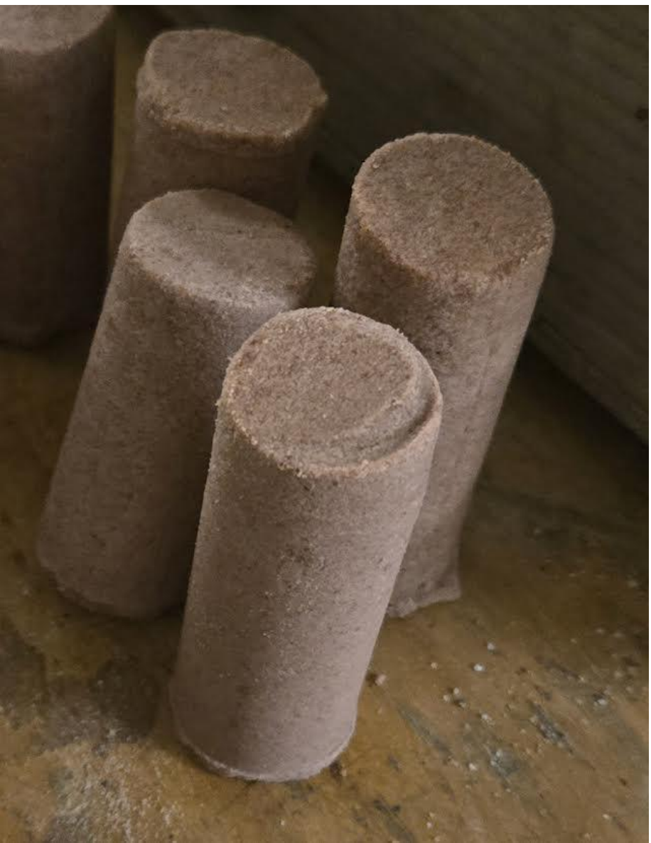
Figure 8: Sandstone cores made from a sample collected at Muddy Mountains, Nevada, USA. Approximately two inches tall.
