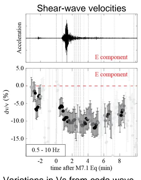
Variations in Vs from coda wave interferometry IRFs in bldg-EW direction from M7.1 Ridgecrest mainshock by applying stretching technique. Grayscale: cross correlation value 0-1. Red dashed line: 225 m/s average from ambient vibration data. Vertical dashed lines show M>4.5 foreshock and aftershock times.
