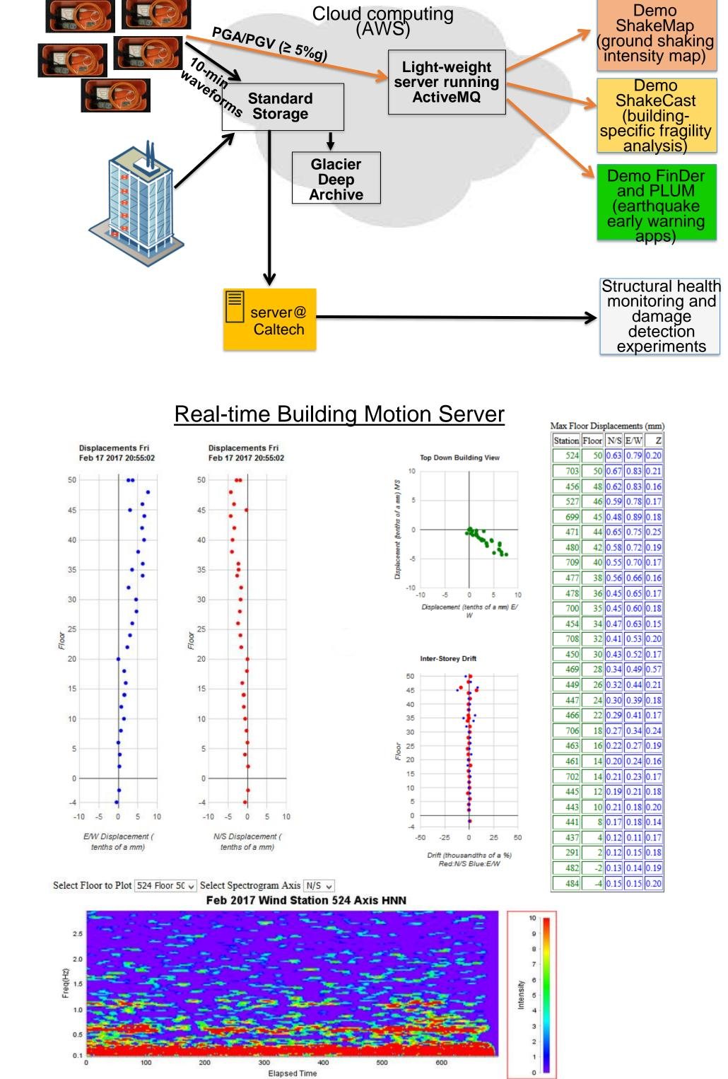
**IoT Seismic Network**
