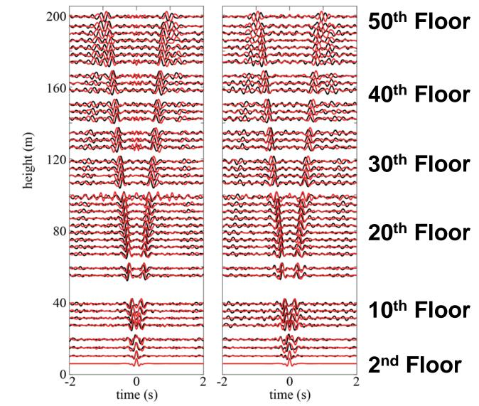
Impulse Response Functions (IRFs) with respect to Floor 2 in 52-story steel moment and brace frame in downtown Los Angeles from ambient vibration data (black traces), and 20-second window during M7.1 Ridgecrest earthquake (red traces) for bldg-EW (Left) and bldg-NS (Right) components from CSN sensors
