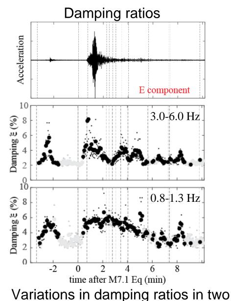
frequency bands from coda wave interferometry IRFs in bldg-EW direction. IRF amplitude envelope decays are measured relative to ambient vibrations. Vertical dashed lines show M>4.5 foreshock and aftershock times. Bldg-NS is similar
