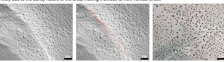
At this location, rupture is not visible on the lidar and lidar artifacts make it hard to reconcile the exact fault locatio In the orthoimagery, while discontinuous, the ruptures are visible and are more easily mapped.
