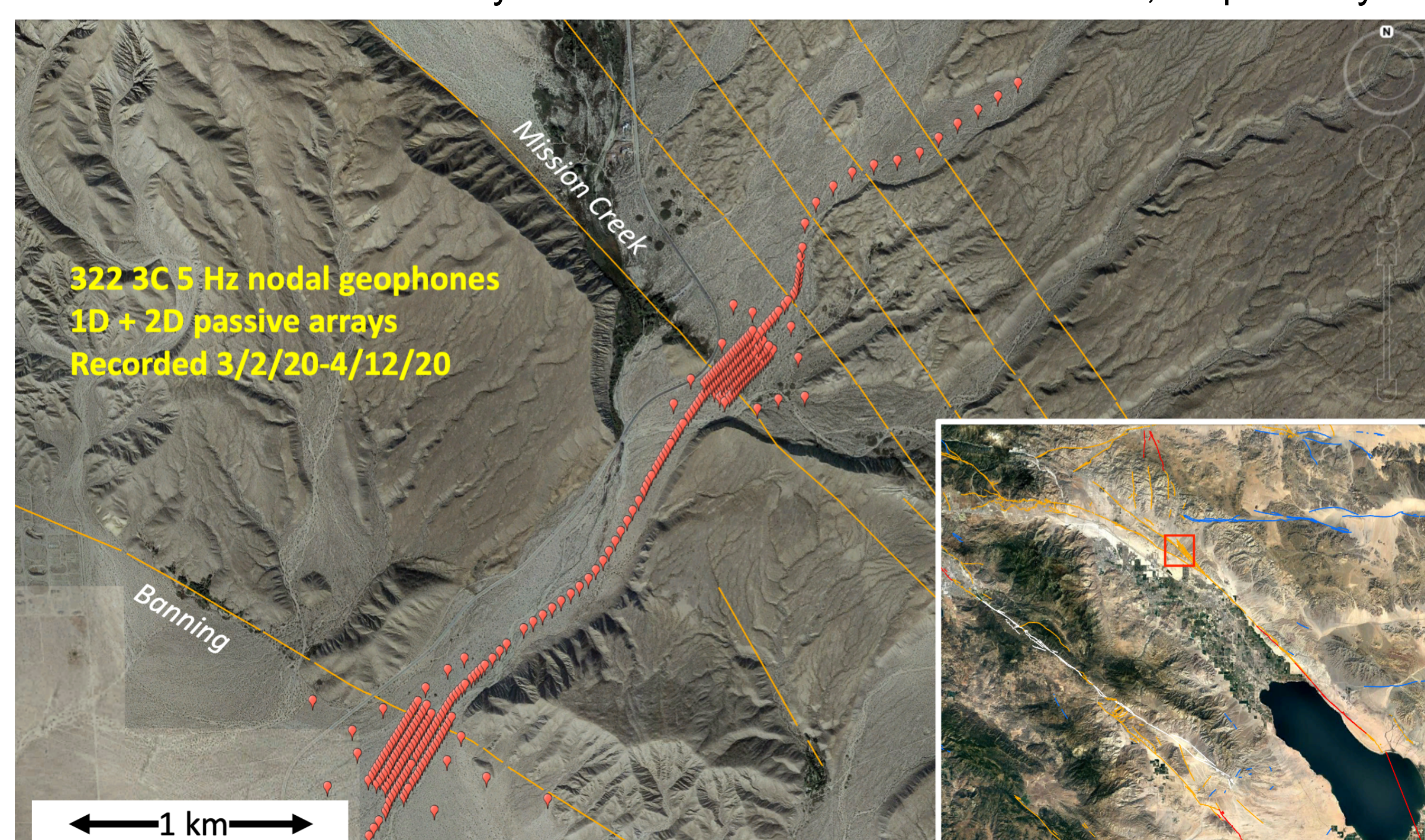
Figure 1: The SSAF Large-N nodal array spanning the merger of the BF and MCF strands around the Thousand Palms Oasis Preserve.
