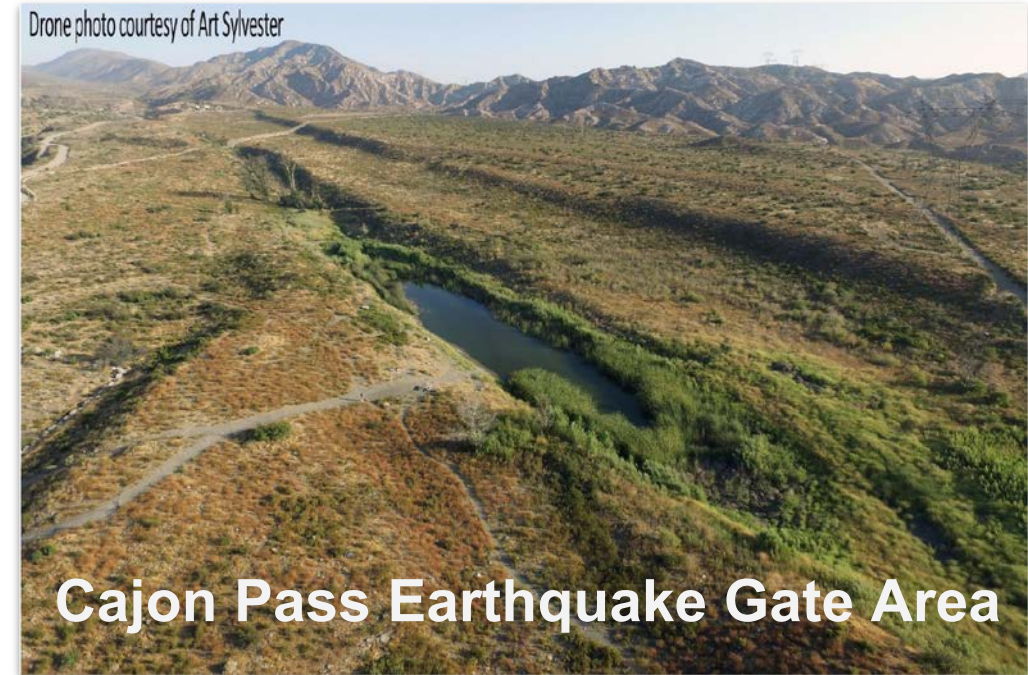
Drone photo (courtesy of Art Sylvester) looking North across the SAF at Lost Lake showing the Lost Lake sag pond, fault scarps, and various terrace risers that were used as piercing lines for determination of slip-rate [Weldon and Sieh, 1985].
