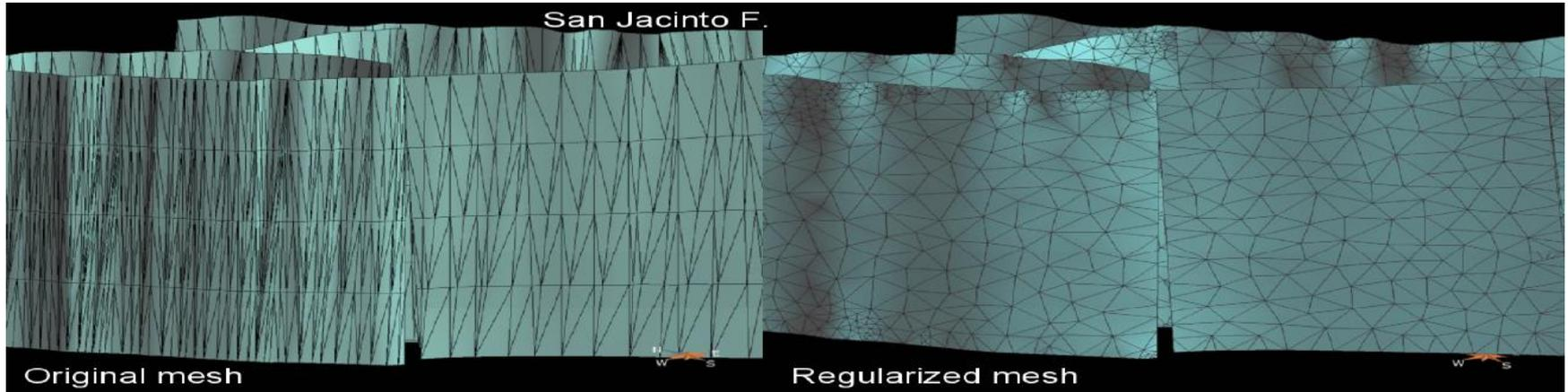
The original CFM4 mesh has lots of long skinny triangles which are bad for simulators.
