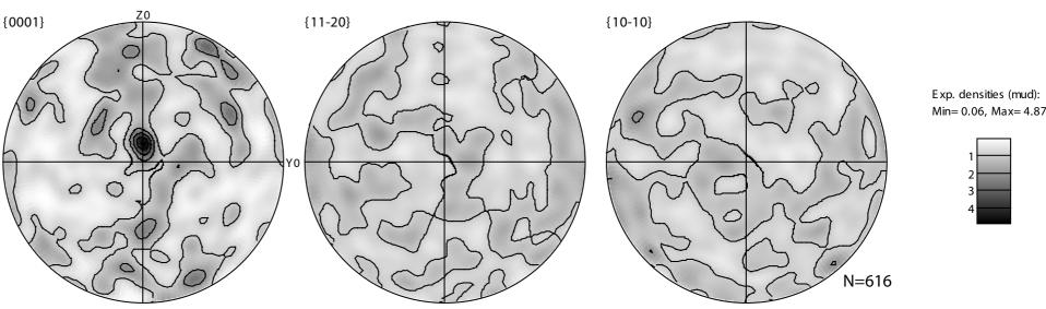
Quartz shows evidence for prism <a> slip, consistent with lower amphibolite facies metamorphism
