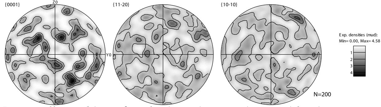
No crystallographic preferred orientation; consistent with microstructural evidence for diffusive mass transfer, grain boundary sliding
