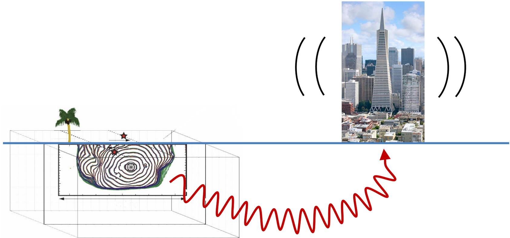
One possible application is a “rupture to rafters” simulation that includes nucleation, rupture propagation, seismic waves, site effects, *and* the shaking of the building and the effects of that shaking on the building systems?
