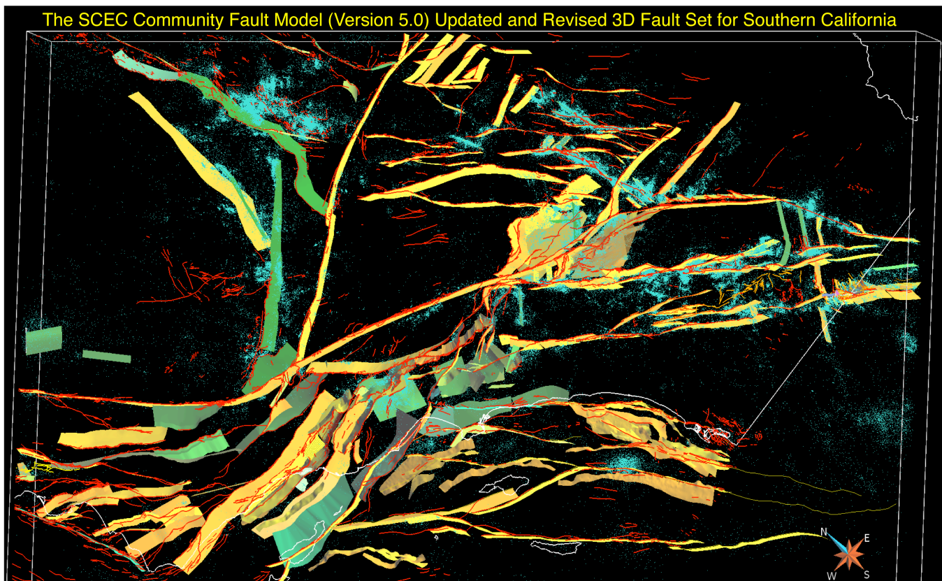
Figure 1. Oblique view looking NE of 2015 CFM-v5 fault models, plus Qfault surface traces (red lines), and relocated seismicity (blue dots) [Nicholson et al. , 2015; Plesch et al. , 2015]. CFM-v5 improvements include 210 new or updated 3D fault models added to CFM since the release of CFM-v4, or a total of over 360 new or updated faults (orange to yellow surfaces) or alternative representations added to CFM since version 3.0, and to the remaining CFM-v3 fault models (green surfaces). Seismicity (1981-2012) from Hauksson et al. [2012].
