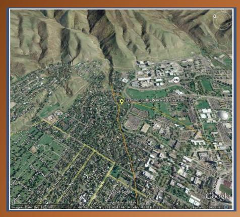
Oblique Google Earth view of the Penrose Drive trench site in northeast Salt Lake Valley. Yellow lines are fault traces from the USGS Quaternary fault-and-fold database.
