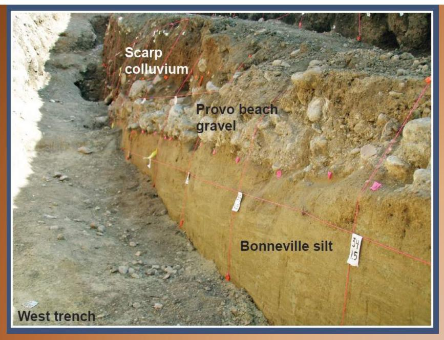
Although the west trench shows flat-lying, undeformed beds, the east trench shows an angular unconformity and tilting (subaqueous faulting?)
