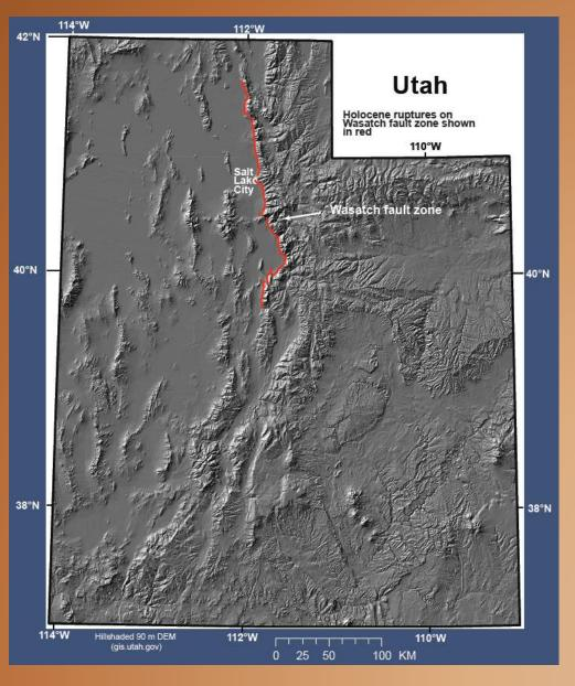
Map of Utah showing extent of Holocene ruptures on the five central segments of the Wasatch fault zone.
